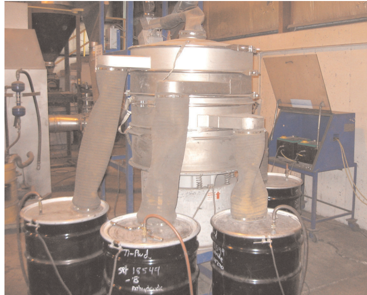
The Russell Vibrasonic Deblinding System being used at the Reading Alloy plant, with their existing screener
