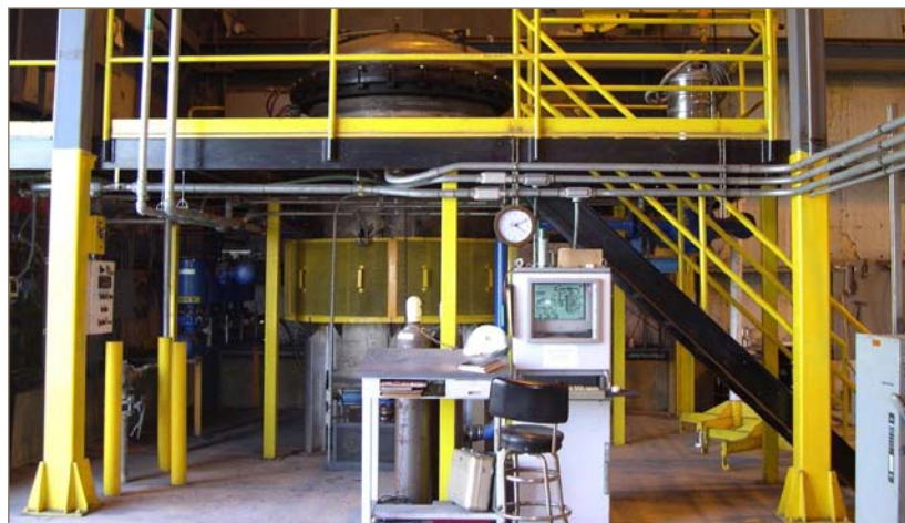
Fig. 2 RAI's production HDH unit.
