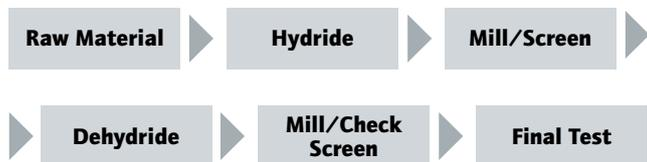
Hydride-Dehydride Process Flow Diagram.
